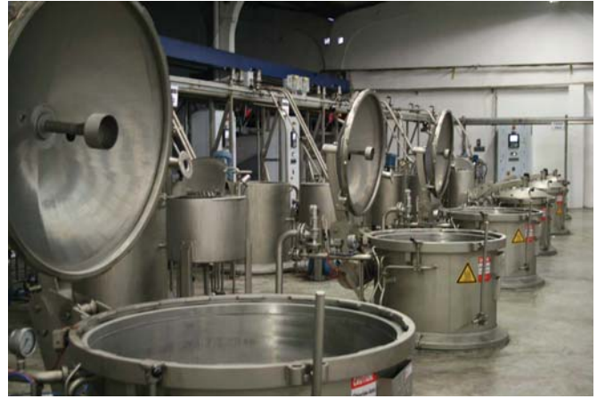
Gülle's dyeing plant houses machines varying in capacity from an hourly 25kg up to 600kg.
